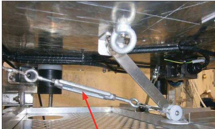
Turnbuckle to adjust cable's length
