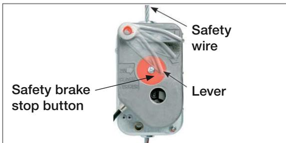
**Step 5 - (Technician 2)** - Releases slowly the handle until the counterweights reach its operational position so that the safety wire rope gets tension again.
